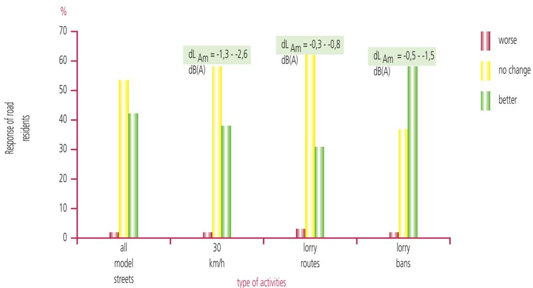
The actions resulted in reductions in average sound levels ranging from 0.3 dB(A) to 2.6 dB(A). The greatest reductions in the average sound level were achieved by speed limits, while the smallest reductions were the result of recommended lorry routes. The effects of the lorry bans fell between the other measures.
