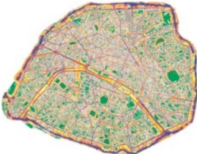
The computation is based on a combination of noise prediction software and a geographical information system. The data comes from several databases that provide three kinds of information: topography, traffic, density of inhabitants.
